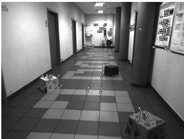
Fig. 3 Scene image and optical flow vectors of the keypoints indicated by white line segments.
