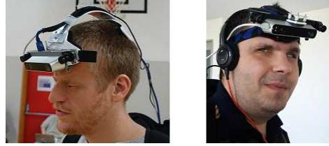
Figure 1: Acquisition devices support attached to different headgear designs. (Left) Rigid acrylic structure resembling VR headset implementations. (Right) Lightweight headgear with elastic strap bands.
