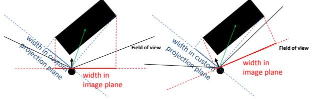
Figure 3: Computing the width of an object based on its projection on the camera plane (red) and custom plane (blue). The width computed with the proposed method (blue) is constant when variating the camera orientation from the same user position.
