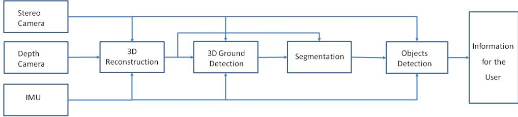
Figure 2: Main processing steps of the proposed system. The functionality and implementation of each step depends on the type of sensed environment (indoor vs. outdoor) and lighting conditions.
