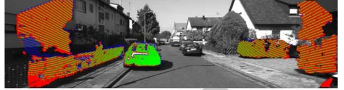
Fig. 7. Obstacles detection results for the KITTI dataset: overlaid segmentation results obtained in both  $\theta$  and U-disparity images
