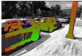
Fig. 11. Obstacles detection results for the virtual environment dataset: overlaid segmentation results obtained in both  $\theta$  and U-disparity images
