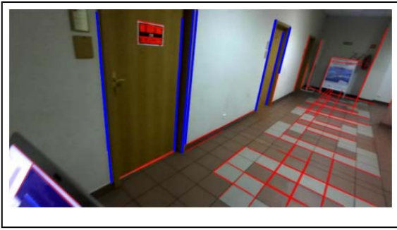
Fig. 8. Door detection example. The detection is performed in indoor scenes based on the fusion of depth and color data coming from the structured light sensor and the stereo vision system, respectively.
